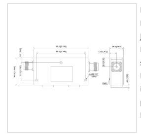
RF Solution offer a wide selection of Dual Junction Isolator for global customers. UIYCDI9648A is a Dual Junction Isolator in Frequency Range of 250~1300 MHz. It is made of high quality materials under a high standard, the Bandwidth Max of this product is 30%, Insertion Loss Max is 0.50~1.60 dB and Isolation Min is 32.0~50.0 dB. The component has a good working performance and stability, it is ideal for handling a Forward Power of 100/300/400 W.
