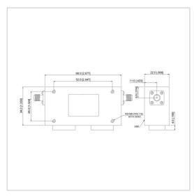
RF Solution offer a wide selection of Dual Junction Isolator for global customers. UIYCDI6834A is a Dual Junction Isolator in Frequency Range of 700~2000 MHz. It is made of high quality materials under a high standard, the Bandwidth Max of this product is 40%, Insertion Loss Max is 0.60~1.20 dB and Isolation Min is 32.0~45.0 dB. The component has a good working performance and stability, it is ideal for handling a Forward Power of 100/120/200 W.
