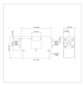
RF Solution offer a wide selection of Dual Junction Isolator for global customers. UIYCDI3928A is a Dual Junction Isolator in Frequency Range of 3.5~7.0 GHz. It is made of high quality materials under a high standard, the Bandwidth Max of this product is 20%, Insertion Loss Max is 0.70~1.00 dB and Isolation Min is 40.0~45.0 dB. The component has a good working performance and stability, it is ideal for handling a Forward Power of 60 W.
