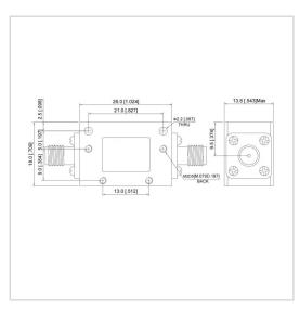
RF Solution offer a wide selection of Dual Junction Isolator for global customers. UIYCDI2618A is a Dual Junction Isolator in Frequency Range of  $6.0\sim27.5$  GHz. It is made of high quality materials under a high standard, the Bandwidth Max of this product is 20%, Insertion Loss Max is  $0.60\sim1.20$  dB and Isolation Min is  $36.0\sim45.0$  dB. The component has a good working performance and stability, it is ideal for handling a Forward Power of 60 W.
