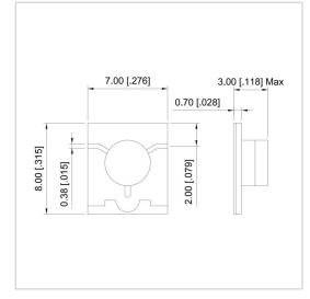
RF Solution offer a wide selection of Microstrip Isolator for global customers. UIYBMI78A is a Microstrip Isolator in Frequency Range of 8.0~12.0 GHz. It is made of high quality materials under a high standard, the Bandwidth Max of this product is 100%, Insertion Loss Max is 0.60 dB and Isolation Min is 18.0 dB. The component has a good working performance and stability, it is ideal for handling a Forward Power of 10 W.
