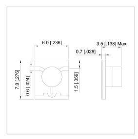
RF Solution offer a wide selection of Microstrip Isolator for global customers. UIYBMI67B is a Microstrip Isolator in Frequency Range of 8.0~12.0 GHz. It is made of high quality materials under a high standard, the Bandwidth Max of this product is 100%, Insertion Loss Max is 0.60 dB and Isolation Min is 17.0 dB. The component has a good working performance and stability, it is ideal for handling a Forward Power of 10 W.
