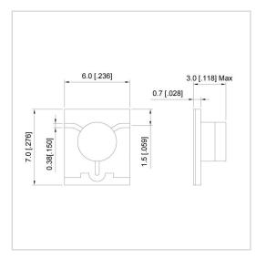
RF Solution offer a wide selection of Microstrip Isolator for global customers. UIYBMI67A is a Microstrip Isolator in Frequency Range of 11.0~18.0 GHz. It is made of high quality materials under a high standard, the Bandwidth Max of this product is 100%, Insertion Loss Max is 0.90 dB and Isolation Min is 15.0 dB. The component has a good working performance and stability, it is ideal for handling a Forward Power of 15 W.
