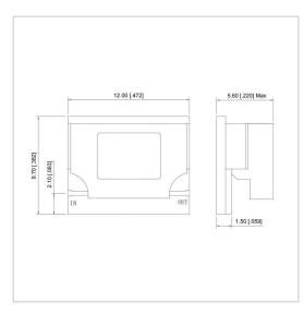
RF Solution offer a wide selection of Microstrip Isolator for global customers. UIYBMI129A is a Microstrip Isolator in Frequency Range of 6.0~18.0 GHz. It is made of high quality materials under a high standard, the Bandwidth Max of this product is 100%, Insertion Loss Max is 1.00~1.30 dB and Isolation Min is 14.0~15.0 dB. The component has a good working performance and stability, it is ideal for handling a Forward Power of 16 W.
