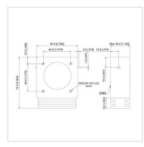
RF Solution offer a wide selection of Drop in Isolator for global customers. UIYBDI6075F is a Drop in Isolator in Frequency Range of 225~400 MHz. It is made of high quality materials under a high standard, the Bandwidth Max of this product is 100%, Insertion Loss Max is 0.80~1.00 dB and Isolation Min is 16.0~18.0 dB. The component has a good working performance and stability, it is ideal for handling a Forward Power of 160 W.
