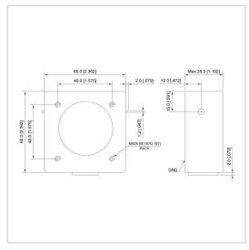
RF Solution offer a wide selection of Drop in Isolator for global customers. UIYBDI6060H is a Drop in Isolator in Frequency Range of 300~475 MHz. It is made of high quality materials under a high standard, the Bandwidth Max of this product is 100%, Insertion Loss Max is 0.80~1.00 dB and Isolation Min is 17.0~18.0 dB. The component has a good working performance and stability, it is ideal for handling a Forward Power of 100 W.
