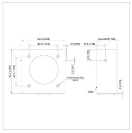
RF Solution offer a wide selection of Drop in Isolator for global customers. UIYBDI6060F is a Drop in Isolator in Frequency Range of 225~400 MHz. It is made of high quality materials under a high standard, the Bandwidth Max of this product is 100%, Insertion Loss Max is 0.80~1.00 dB and Isolation Min is 16.0~18.0 dB. The component has a good working performance and stability, it is ideal for handling a Forward Power of 160 W.
