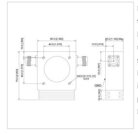
RF Solution offer a wide selection of Coaxial Isolator for global customers. UIYBCI6075F is a Coaxial Isolator in Frequency Range of 225~400 MHz. It is made of high quality materials under a high standard, the Bandwidth Max of this product is 100%, Insertion Loss Max is 0.80~1.00 dB and Isolation Min is 16.0~18.0 dB. The component has a good working performance and stability, it is ideal for handling a Forward Power of 100/160 W.
