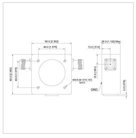
RF Solution offer a wide selection of Coaxial Isolator for global customers. UIYBCI6060H is a Coaxial Isolator in Frequency Range of 300~475 MHz. It is made of high quality materials under a high standard, the Bandwidth Max of this product is 100%, Insertion Loss Max is 0.80~1.00 dB and Isolation Min is 17.0~18.0 dB. The component has a good working performance and stability, it is ideal for handling a Forward Power of 100 W.
