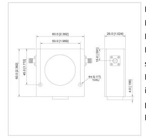
RF Solution offer a wide selection of Broadband Isolator for global customers. UIYBCI6060G is a Broadband Isolator in Frequency Range of 600~900 MHz. It is made of high quality materials under a high standard, the Bandwidth Max of this product is 100%, Insertion Loss Max is 0.50~0.80 dB and Isolation Min is 15.0~16.0 dB. The component has a good working performance and stability, it is ideal for handling a Forward Power of 100 W.
