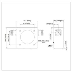
RF Solution offer a wide selection of Coaxial Isolator for global customers. UIYBCI6060F is a Coaxial Isolator in Frequency Range of 225~400 MHz. It is made of high quality materials under a high standard, the Bandwidth Max of this product is 100%, Insertion Loss Max is 0.80~1.00 dB and Isolation Min is 16.0~18.0 dB. The component has a good working performance and stability, it is ideal for handling a Forward Power of 100/160 W.
