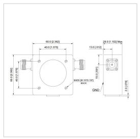
RF Solution offer a wide selection of Broadband Isolator for global customers. UIYBCI6060E is a Broadband Isolator in Frequency Range of 56~86 MHz. It is made of high quality materials under a high standard, the Bandwidth Max of this product is 100%, Insertion Loss Max is 1.50 dB and Isolation Min is 16.0 dB. The component has a good working performance and stability, it is ideal for handling a Forward Power of 60 W.
