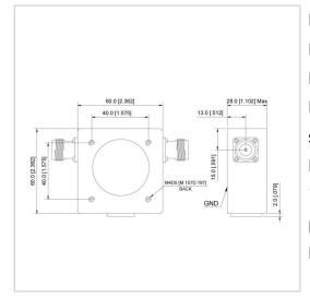
RF Solution offer a wide selection of Broadband Isolator for global customers. UIYBCI6060C is a Broadband Isolator in Frequency Range of 130~180 MHz. It is made of high quality materials under a high standard, the Bandwidth Max of this product is 100%, Insertion Loss Max is 0.80 dB and Isolation Min is 18.0 dB. The component has a good working performance and stability, it is ideal for handling a Forward Power of 100 W.
