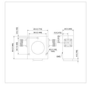
RF Solution offer a wide selection of Broadband Isolator for global customers. UIYBCI4550A is a Broadband Isolator in Frequency Range of 950~1450 MHz. It is made of high quality materials under a high standard, the Bandwidth Max of this product is 100%, Insertion Loss Max is 0.60 dB and Isolation Min is 16.0 dB. The component has a good working performance and stability, it is ideal for handling a Forward Power of 100/200 W.
