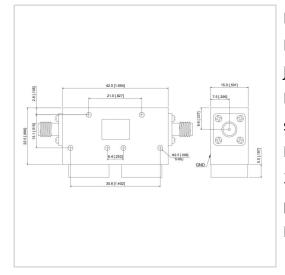
RF Solution offer a wide selection of Dual Junction Isolator for global customers. UIYBCI4222A is a Dual Junction Isolator in Frequency Range of 4.0~8.0 GHz. It is made of high quality materials under a high standard, the Bandwidth Max of this product is 100%, Insertion Loss Max is 1.00 dB and Isolation Min is 36.0 dB. The component has a good working performance and stability, it is ideal for handling a Forward Power of 100 W.
