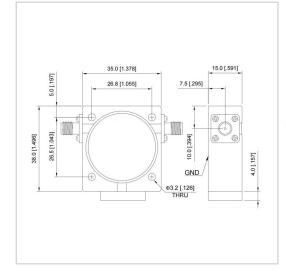
RF Solution offer a wide selection of Broadband Isolator for global customers. UIYBCI3538B is a Broadband Isolator in Frequency Range of 400~470 MHz. It is made of high quality materials under a high standard, the Bandwidth Max of this product is 100%, Insertion Loss Max is 0.40 dB and Isolation Min is 20.0 dB. The component has a good working performance and stability, it is ideal for handling a Forward Power of 300/100 W.
