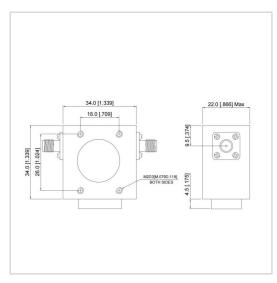
RF Solution offer a wide selection of Broadband Isolator for global customers. UIYBCI3434F is a Broadband Isolator in Frequency Range of 1225~1875 MHz. It is made of high quality materials under a high standard, the Bandwidth Max of this product is 100%, Insertion Loss Max is 0.60 dB and Isolation Min is 16.0 dB. The component has a good working performance and stability, it is ideal for handling a Forward Power of 100/200 W.
