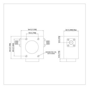
RF Solution offer a wide selection of Broadband Isolator for global customers. UIYBCI3434D is a Broadband Isolator in Frequency Range of 950~1415 MHz. It is made of high quality materials under a high standard, the Bandwidth Max of this product is 100%, Insertion Loss Max is 0.60 dB and Isolation Min is 18.0 dB. The component has a good working performance and stability, it is ideal for handling a Forward Power of 100/200 W.
