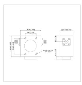
RF Solution offer a wide selection of Broadband Isolator for global customers. UIYBCI3434A is a Broadband Isolator in Frequency Range of 800~1000 MHz. It is made of high quality materials under a high standard, the Bandwidth Max of this product is 100%, Insertion Loss Max is 0.40 dB and Isolation Min is 20.0 dB. The component has a good working performance and stability, it is ideal for handling a Forward Power of 100/200 W.
