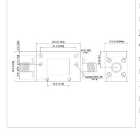
RF Solution offer a wide selection of Dual Junction Isolator for global customers. UIYBCI2618B is a Dual Junction Isolator in Frequency Range of 12.0~18.0 GHz. It is made of high quality materials under a high standard, the Bandwidth Max of this product is 100%, Insertion Loss Max is 1.00 dB and Isolation Min is 36.0 dB. The component has a good working performance and stability, it is ideal for handling a Forward Power of 60 W.
