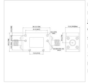
RF Solution offer a wide selection of Dual Junction Isolator for global customers. UIYBCI2618A is a Dual Junction Isolator in Frequency Range of 8.0~12.0 GHz. It is made of high quality materials under a high standard, the Bandwidth Max of this product is 100%, Insertion Loss Max is 1.00 dB and Isolation Min is 36.0 dB. The component has a good working performance and stability, it is ideal for handling a Forward Power of 60 W.
