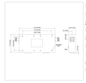
RF Solution offer a wide selection of Dual Junction Isolator for global customers. UIYBCI14272A is a Dual Junction Isolator in Frequency Range of 1.0~2.0 GHz. It is made of high quality materials under a high standard, the Bandwidth Max of this product is 100%, Insertion Loss Max is 1.40 dB and Isolation Min is 34.0 dB. The component has a good working performance and stability, it is ideal for handling a Forward Power of 100/300 W.
