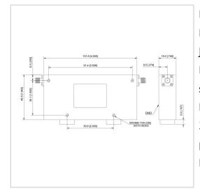
RF Solution offer a wide selection of Dual Junction Isolator for global customers. UIYBCI10149B is a Dual Junction Isolator in Frequency Range of 1.5~3.0 GHz. It is made of high quality materials under a high standard, the Bandwidth Max of this product is 100%, Insertion Loss Max is 1.00 dB and Isolation Min is 34.0 dB. The component has a good working performance and stability, it is ideal for handling a Forward Power of 100 W.
