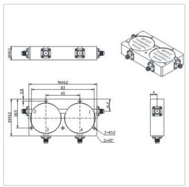
RF Solution offer a wide selection of Dual Junction Circulator for global customers. THH9050XS is a Dual Junction Circulator in Frequency Range of 300-1400 MHz. It is made of high quality materials under a high standard, the Bandwidth Max of this product is 20%, Insertion Loss Max is 1.7 dB and Isolation Min is 30.0 dB. The component has a good working performance and stability, it is ideal for handling a Forward Power of 100 W.
