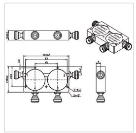
RF Solution offer a wide selection of Dual Junction Circulator for global customers. THH9050XN is a Dual Junction Circulator in Frequency Range of 300-1250 MHz. It is made of high quality materials under a high standard, the Bandwidth Max of this product is 20%, Insertion Loss Max is 1.7 dB and Isolation Min is 30.0 dB. The component has a good working performance and stability, it is ideal for handling a Forward Power of 100 W.
