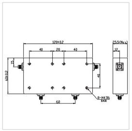
RF Solution offer a wide selection of Dual Junction Circulator for global customers. THH12060ES is a Dual Junction Circulator in Frequency Range of 80-230 MHz. It is made of high quality materials under a high standard, the Bandwidth Max of this product is 30%, Insertion Loss Max is 2.2 dB and Isolation Min is 36.0 dB. The component has a good working performance and stability, it is ideal for handling a Forward Power of 100W.
