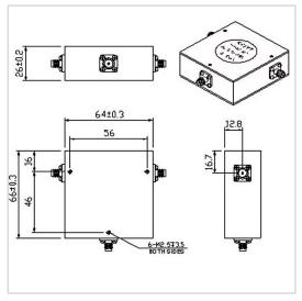
RF Solution offer a wide selection of Coaxial Circulator for global customers. TH6466KS is a Coaxial Circulator in Frequency Range of 950~2000 MHz. It is made of high quality materials under a high standard, the Bandwidth Max of this product is 100%, Insertion Loss Max is 0.70~0.80 dB and Isolation Min is 16.0~17.0 dB. The component has a good working performance and stability, it is ideal for handling a Forward Power of 100 W.
