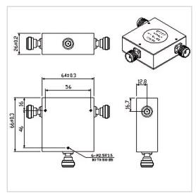
RF Solution offer a wide selection of Coaxial Circulator for global customers. TH6466KN is a Coaxial Circulator in Frequency Range of 950~2000 MHz. It is made of high quality materials under a high standard, the Bandwidth Max of this product is 100%, Insertion Loss Max is 0.70~0.80 dB and Isolation Min is 16.0~17.0 dB. The component has a good working performance and stability, it is ideal for handling a Forward Power of 150 W.
