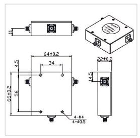
RF Solution offer a wide selection of Coaxial Circulator for global customers. TH6466HS is a Coaxial Circulator in Frequency Range of 30~40 MHz. It is made of high quality materials under a high standard, the Bandwidth Max of this product is 5%, Insertion Loss Max is 1.50~2.00 dB and Isolation Min is 18.0~20.0 dB. The component has a good working performance and stability, it is ideal for handling a Forward Power of 100 W.
