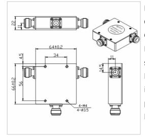
RF Solution offer a wide selection of Coaxial Circulator for global customers. TH6466HN is a Coaxial Circulator in Frequency Range of 30~40 MHz. It is made of high quality materials under a high standard, the Bandwidth Max of this product is 5%, Insertion Loss Max is 1.50~2.00 dB and Isolation Min is 18.0~20.0 dB. The component has a good working performance and stability, it is ideal for handling a Forward Power of 100 W.
