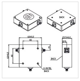
RF Solution offer a wide selection of Coaxial Circulator for global customers. TH6060ES is a Coaxial Circulator in Frequency Range of 30~400 MHz. It is made of high quality materials under a high standard, the Bandwidth Max of this product is 50%, Insertion Loss Max is 0.50~1.80 dB and Isolation Min is 18.0~23.0 dB. The component has a good working performance and stability, it is ideal for handling a Forward Power of 100 W.
