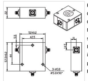
RF Solution offer a wide selection of Coaxial Circulator for global customers. TH5258ES is a Coaxial Circulator in Frequency Range of 160~300 MHz. It is made of high quality materials under a high standard, the Bandwidth Max of this product is 20%, Insertion Loss Max is 0.50~1.80 dB and Isolation Min is 18.0~23.0 dB. The component has a good working performance and stability, it is ideal for handling a Forward Power of 100 W.
