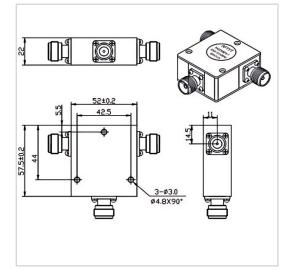
RF Solution offer a wide selection of Coaxial Circulator for global customers. TH5258EN is a Coaxial Circulator in Frequency Range of 160~300 MHz. It is made of high quality materials under a high standard, the Bandwidth Max of this product is 20%, Insertion Loss Max is 0.50~1.80 dB and Isolation Min is 18.0~23.0 dB. The component has a good working performance and stability, it is ideal for handling a Forward Power of 500 W.
