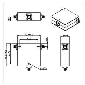
RF Solution offer a wide selection of Coaxial Circulator for global customers. TH5050AS is a Coaxial Circulator in Frequency Range of 1.25~3.0 GHz. It is made of high quality materials under a high standard, the Bandwidth Max of this product is 100%, Insertion Loss Max is 0.70~0.80 dB and Isolation Min is 16.0~17.0 dB. The component has a good working performance and stability, it is ideal for handling a Forward Power of 100 W.
