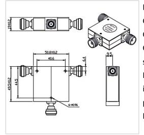
RF Solution offer a wide selection of Coaxial Circulator for global customers. TH5050AN is a Coaxial Circulator in Frequency Range of 1.25~3.0 GHz. It is made of high quality materials under a high standard, the Bandwidth Max of this product is 100%, Insertion Loss Max is 0.70~0.80 dB and Isolation Min is 16.0~17.0 dB. The component has a good working performance and stability, it is ideal for handling a Forward Power of 100 W.
