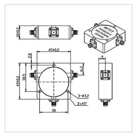
RF Solution offer a wide selection of Coaxial Circulator for global customers. TH4550XS is a Coaxial Circulator in Frequency Range of 250~1400 MHz. It is made of high quality materials under a high standard, the Bandwidth Max of this product is 40%, Insertion Loss Max is 0.30~0.80 dB and Isolation Min is 18.0~23.0 dB. The component has a good working performance and stability, it is ideal for handling a Forward Power of 100 W.
