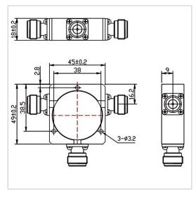
RF Solution offer a wide selection of Coaxial Circulator for global customers. TH4550XN is a Coaxial Circulator in Frequency Range of 250~1400 MHz. It is made of high quality materials under a high standard, the Bandwidth Max of this product is 40%, Insertion Loss Max is 0.30~0.80 dB and Isolation Min is 18.0~25.0 dB. The component has a good working performance and stability, it is ideal for handling a Forward Power of 300 W.
