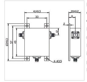
RF Solution offer a wide selection of Coaxial Circulator for global customers. TH4149AS is a Coaxial Circulator in Frequency Range of 300~1000 MHz. It is made of high quality materials under a high standard, the Bandwidth Max of this product is 50%, Insertion Loss Max is 0.60~1.20 dB and Isolation Min is 16.0~20.0 dB. The component has a good working performance and stability, it is ideal for handling a Forward Power of 100 W.
