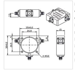
RF Solution offer a wide selection of Coaxial Circulator for global customers. TH3538XS is a Coaxial Circulator in Frequency Range of 300~1850 MHz. It is made of high quality materials under a high standard, the Bandwidth Max of this product is 30%, Insertion Loss Max is 0.20~0.60 dB and Isolation Min is 17.0~25.0 dB. The component has a good working performance and stability, it is ideal for handling a Forward Power of 100 W.
