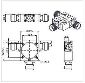
RF Solution offer a wide selection of Coaxial Circulator for global customers. TH3538XN is a Coaxial Circulator in Frequency Range of 300~1850 MHz. It is made of high quality materials under a high standard, the Bandwidth Max of this product is 30%, Insertion Loss Max is 0.20~0.80 dB and Isolation Min is 16.0~25.0 dB. The component has a good working performance and stability, it is ideal for handling a Forward Power of 100 W.
