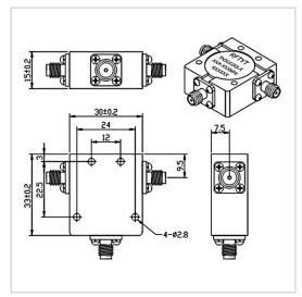
RF Solution offer a wide selection of Coaxial Circulator for global customers. TH3033XS is a Coaxial Circulator in Frequency Range of 700~3000 MHz. It is made of high quality materials under a high standard, the Bandwidth Max of this product is 25%, Insertion Loss Max is 0.30~0.60 dB and Isolation Min is 18.0~23.0 dB. The component has a good working performance and stability, it is ideal for handling a Forward Power of 100 W.
