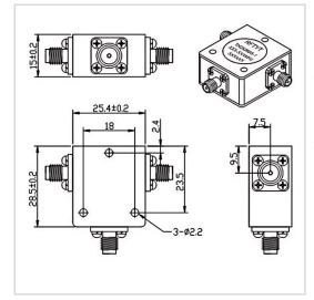
RF Solution offer a wide selection of Coaxial Circulator for global customers. TH2528XS-2222 is a Coaxial Circulator in Frequency Range of 700~5000 MHz. It is made of high quality materials under a high standard, the Bandwidth Max of this product is 25%, Insertion Loss Max is 0.15~0.60 dB and Isolation Min is 16.0~25.0 dB. The component has a good working performance and stability, it is ideal for handling a Forward Power of 100 W.
