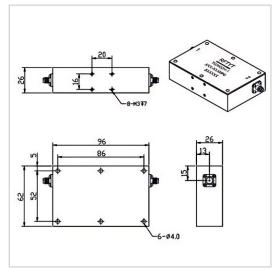
RF Solution offer a wide selection of Dual Junction Isolator for global customers. TG9662HS is a Dual Junction Isolator in Frequency Range of  $300\sim1250$  MHz. It is made of high quality materials under a high standard, the Bandwidth Max of this product is  $5\sim20\%$ , Insertion Loss Max is  $0.50\sim1.20$  dB and Isolation Min is  $34.0\sim50.0$  dB. The component has a good working performance and stability, it is ideal for handling a Forward Power of 100~W.
