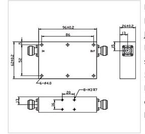
RF Solution offer a wide selection of Dual Junction Isolator for global customers. TG9662HN is a Dual Junction Isolator in Frequency Range of 80~230 MHz. It is made of high quality materials under a high standard, the Bandwidth Max of this product is 5~20%, Insertion Loss Max is 0.50~1.60 dB and Isolation Min is 35.0~50.0 dB. The component has a good working performance and stability, it is ideal for handling a Forward Power of 100 W.
