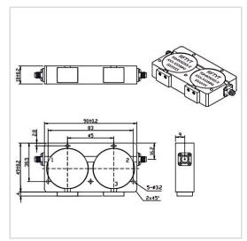
RF Solution offer a wide selection of Dual Junction Isolator for global customers. TG9050XS is a Dual Junction Isolator in Frequency Range of  $300\sim1250$  MHz. It is made of high quality materials under a high standard, the Bandwidth Max of this product is  $5\sim20\%$ , Insertion Loss Max is  $0.50\sim1.60$  dB and Isolation Min is  $32.0\sim50.0$  dB. The component has a good working performance and stability, it is ideal for handling a Forward Power of 100~W.
