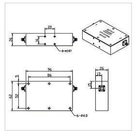
RF Solution offer a wide selection of Dual Junction Isolator for global customers. TG9050XN is a Dual Junction Isolator in Frequency Range of  $300\sim1250$  MHz. It is made of high quality materials under a high standard, the Bandwidth Max of this product is  $5\sim20\%$ , Insertion Loss Max is  $0.50\sim1.60$  dB and Isolation Min is  $32.0\sim50.0$  dB. The component has a good working performance and stability, it is ideal for handling a Forward Power of 100~W.
